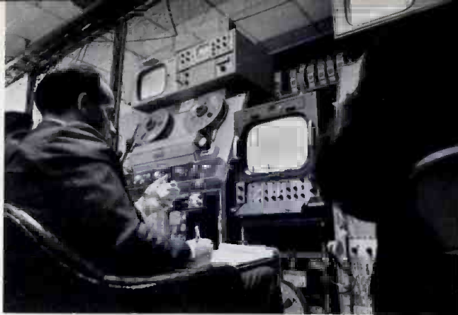
Fig. 2 A typical Olympic setup for electronic editing of daily events into completed evening program for transmission. Conrac monitors are used in this shot for picture quality control.
